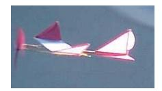
The DennyDart MarkII is a balsa stick & tissue model airplane that is suitable for 12 yr olds and up. It is an easy to build and fly rubber powered model that can be flown either indoor (school gym) or outdoors in calm conditions. It will fly many hundreds of feet so a large open space is needed. As a razor blade is needed, adult supervision is recommenced.
