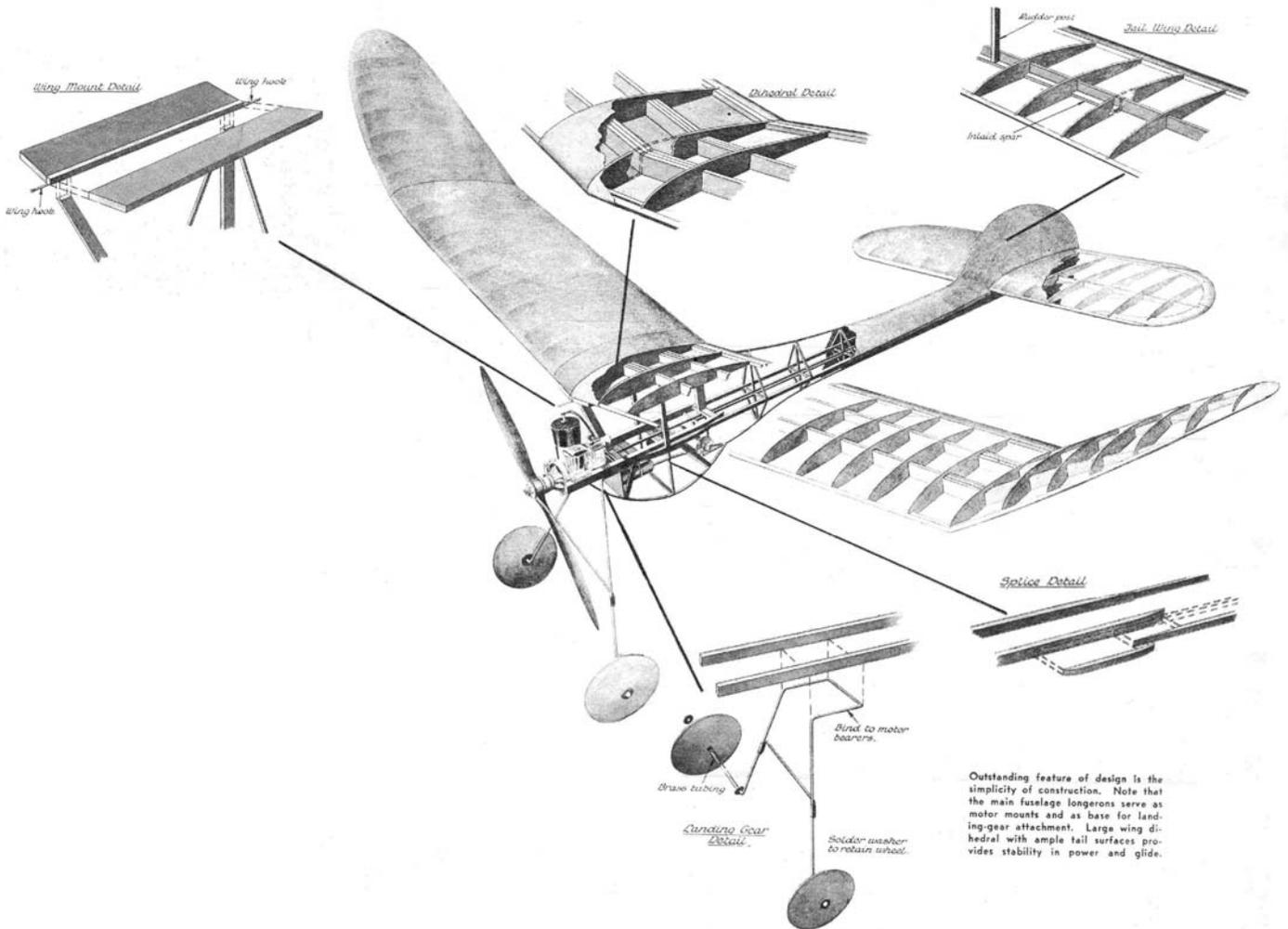
Outstanding feature of design is the simplicity of construction. Note that the main fuselage longerons serve as motor mounts and as base for landing-gear attachment. Large wing dihedral with ample tail surfaces provides stability in power and glide.
