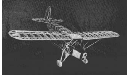
Skeleton of the Ranger ready for covering.
