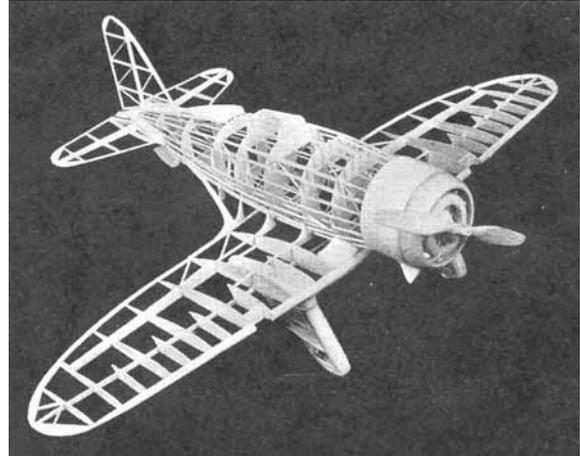
The framework of the Seversky 3-L before covering. Note the fairing strips on the fuselage and the short sub-ribs in the wing construction.
