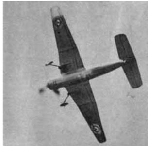
Plenty of wing area, light but sturdy construction, and a long rubber motor spell performance. Many flights of two minutes have been made.
