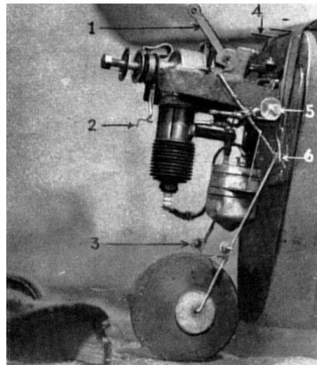
1-timer, 2-spark extension, 3-cowling retainers, 4-cowling pins, 5-throttle, 6-wing hooks. Nose cowling is quickly detachable.
