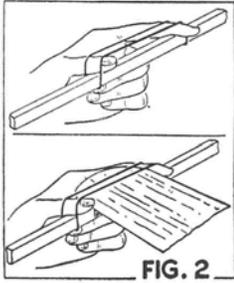
With the assembly of the motors completed, we have only to add the wing and elevator to our A-frame to complete the job. Both these units are held with rubber bands. Two bands are used for each. Note how this is done in Fig. 2. Locate the trailing edge of the wing 6" from the trailing ends of the sticks and
